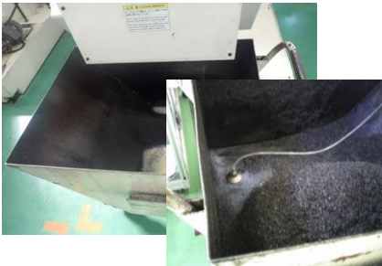
Coolant accumulated in the chip truck is circulated through the liquid connector and used.
