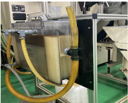
Reduction in the number of cutting fluid changes by installing oil-skimming equipment
