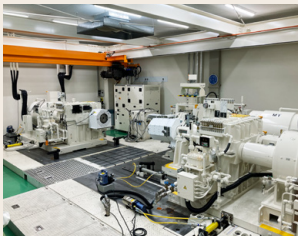
Advanced testing equipment (Three-Wheel Dynamometer)
