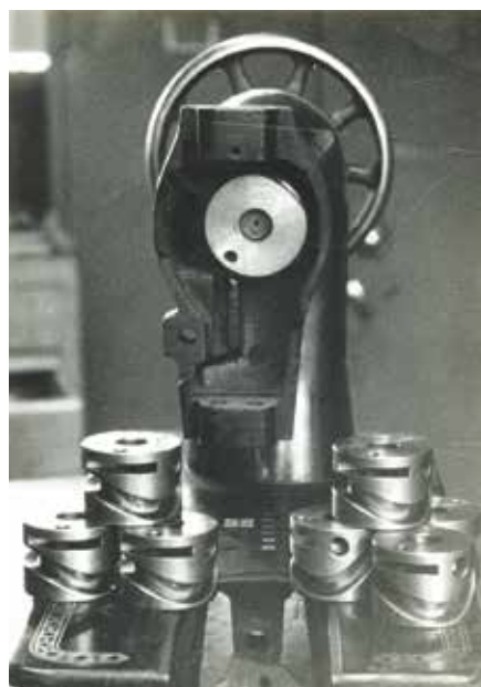
Thread take-up cams and side view in sewing machine
