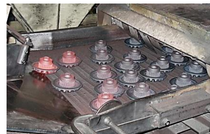
Materials on the Mesh Belt to the Normalizing Furnace
