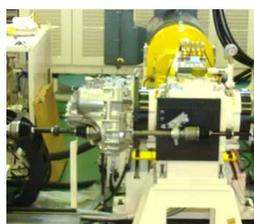
Vehicle Mock Test with 3-axis Dynamo Tester
